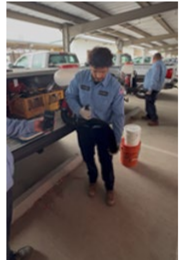
Field staff performing calibrations to backpacks and handheld liquid applications. This is conducted annually to ensure applications are done according to the label.
