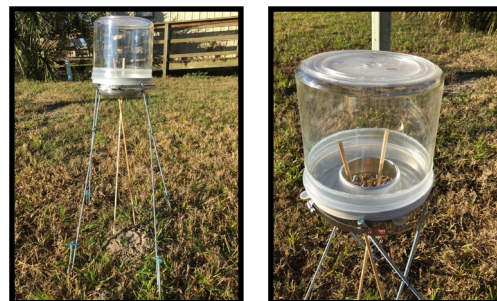
Fig. 2. Redesigned fire ant alate trap with dowel rods that guide alates into a collecting pan. Alates typically crawl to a high perch when they initiate mating flights.
