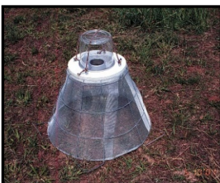
Fig. 1 Previous fire ant alate trap with inverted wire basket and screening that funnels alates initiating flights into a pan filled with collecting fluid.
