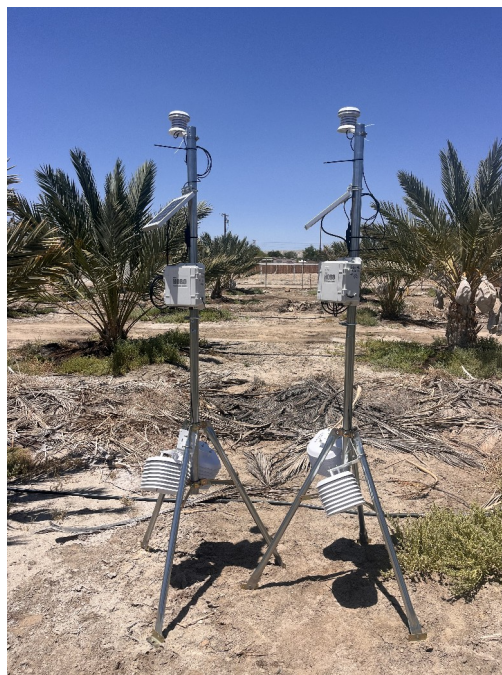
Figure 2. Initial deployment of the field weather station network used to validate remotely sensed environmental data.
