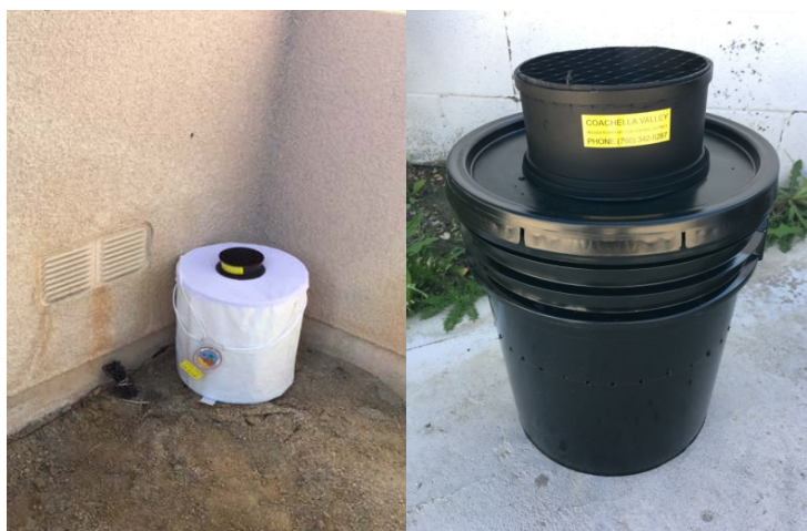
Left: BG Sentinel trap. Right: Autocidal Gravid Trap (AGO).
