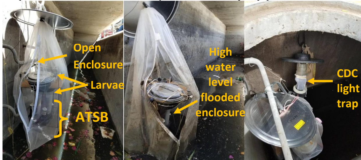
Figure 1. Open portable mesh enclosures for field assessment of ATSBs in USDS in the Coachella Valley. Note the water levels at the same site (Coachella-A2) at day 1 (left) and day 20 (center) of the USDS trial.
