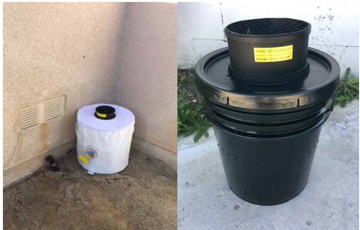
Left: BG Sentinel trap. Right: Autocidal Gravid Trap (AGO).
